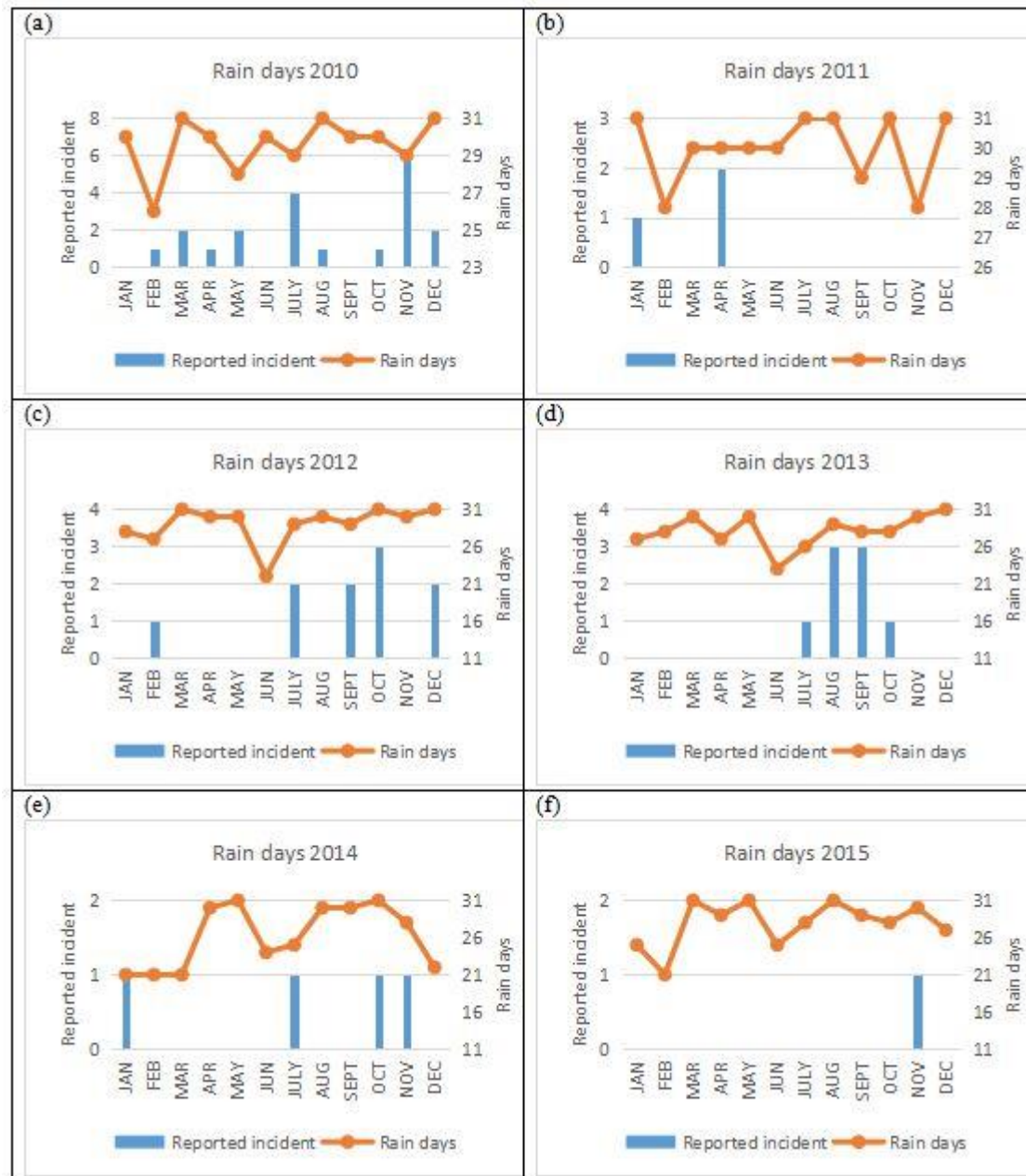
Figure 5. Graph of landslide incidents reported in Kuala Lumpur against rain days from year 2010 to 2015
