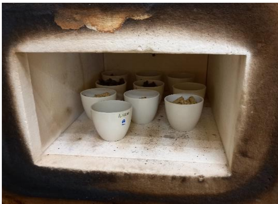
Figure 2 The sample were placed into the muffle furnace for burning process to collect the dry ash remained.
