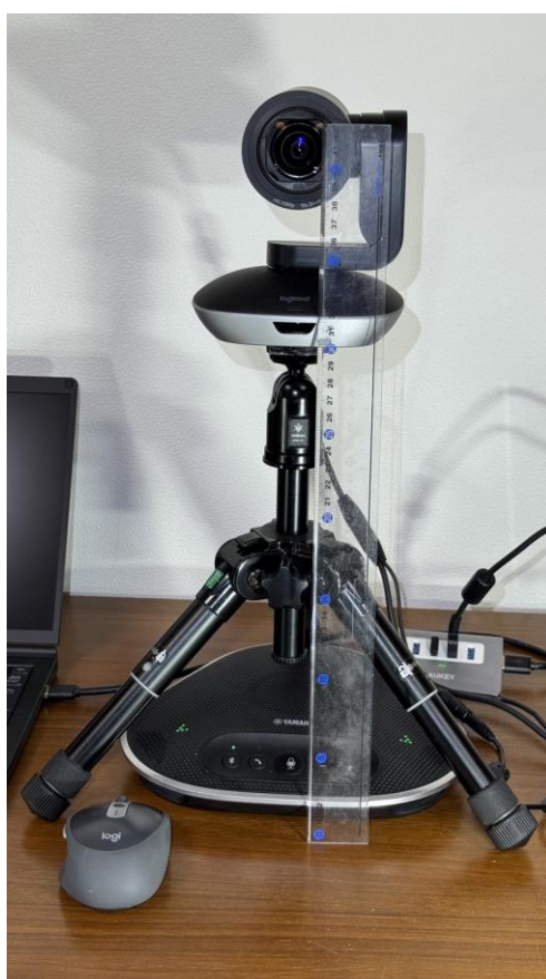
Figure 1 The preliminary system in place. The PTZ camera stands on a tabletop tripod that straddles the speakerphone, so that the camera and microphone share a single footprint on the desk
