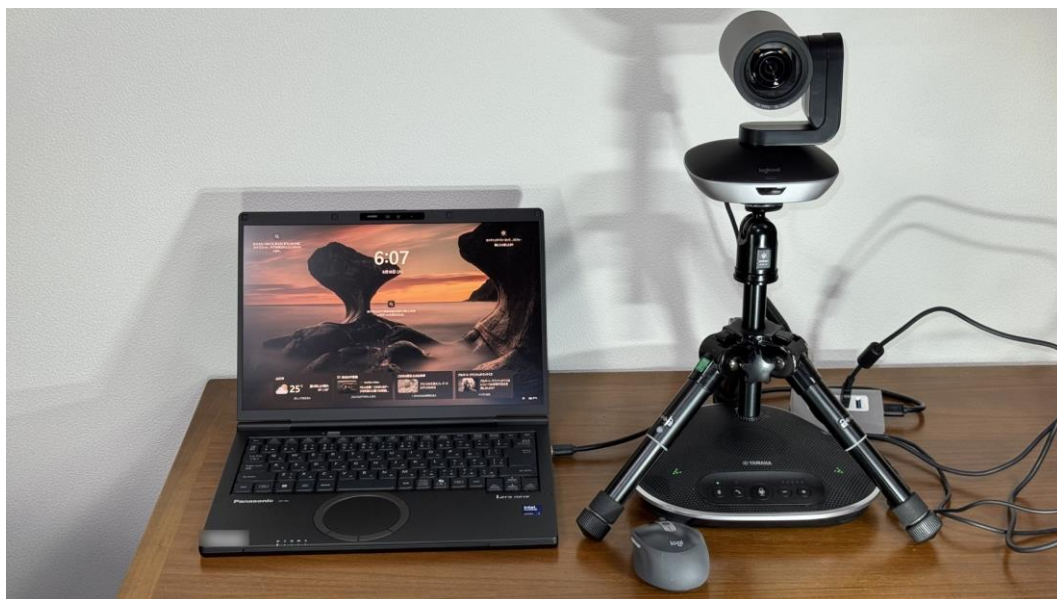
Figure 1 The preliminary system in place. The PTZ camera stands on a tabletop tripod that straddles the speakerphone, so that the camera and microphone share a single footprint on the desk
