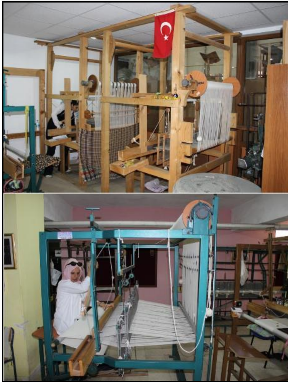
Photo 1. Wooden and metal handlooms with whips where Rize fabric is woven
