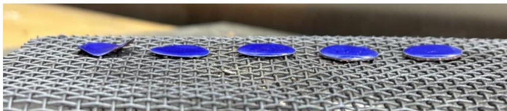
(Figure10) Deformation Resistance Firing Experiment Diagram 2 of Red Copper Samples Image source: Photographed by the author.
