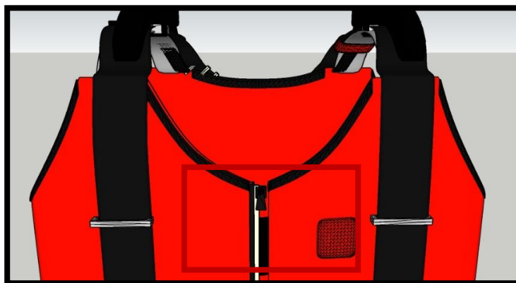
Figure 4.12: The position of heartbeat sensor fiber textiles in passive skeletal safety jacket
