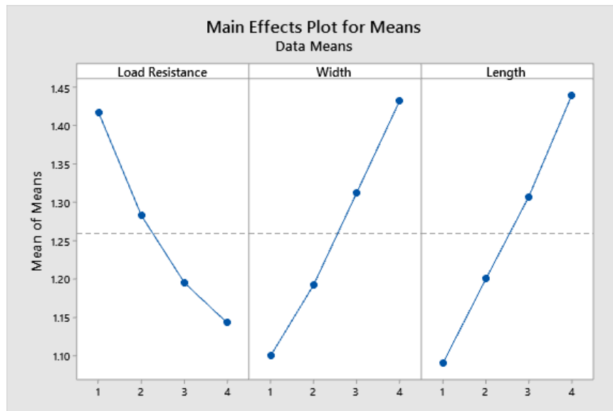
Figure 6 Graph of main effects plot for means electrical power versus load, width, and length
