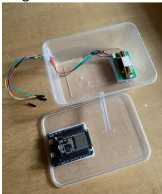
Figure 5: Prototype of the IoT-enabled breath sensor system
