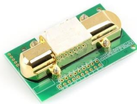
Figure 2: MH-Z14A non-dispersive infrared gas sensor
