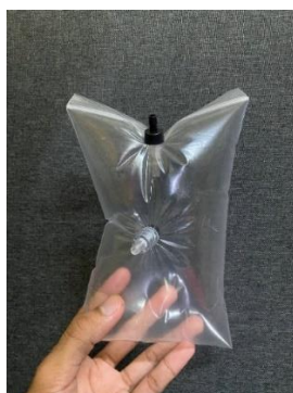
Figure 6: DIY Tedlar bag for breath sample collection
