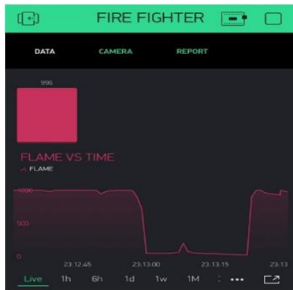
Fig. 6: Live data from flame sensor before and after fire extinguishment.
