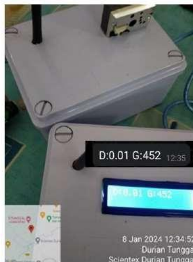
Figure 13: LCD screen and Telegram notification when gas is detected
