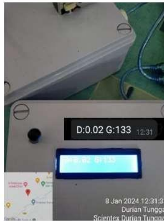
Figure 12: LCD screen and Telegram notification when gas no detected
