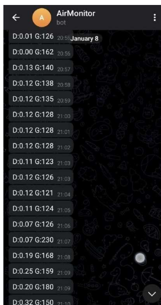
Figure 18: Telegram bot display for PM2.5 and smoke detected by dust sensor
