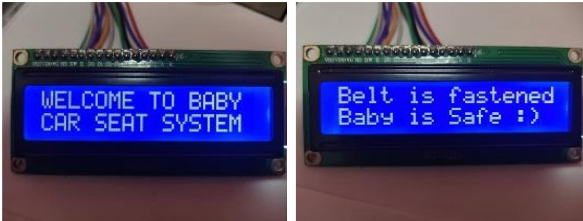
Figure 8 left: LCD shows at start up, right- ,LCD shows status when the seat belt is fastened
