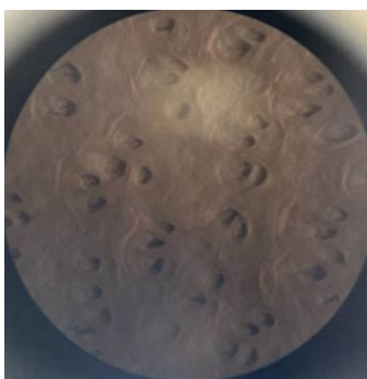
Figure 2: Vegetable-tanned cow leather surface using Binocular Microscope with 10x magnification.
