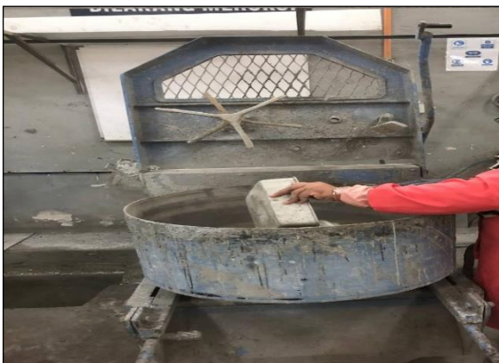
(g) Mix for Base Lining Using Concrete Mixer
