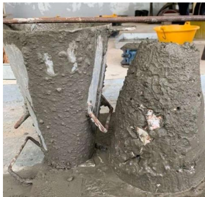
Figure 3: The result of the Slump Test
