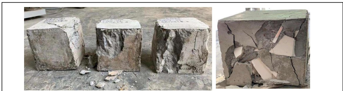
Figure 5: Samples of the normal concrete and CTA concrete specimens after running The Compressive Strength Test
